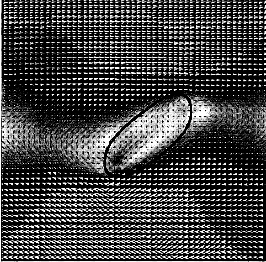
Figure 7. Close-up of relative velocity vectors in the x - y plane with q_{rel} in the background at Re_B \sim 11 corresponding to t = 15 for (a) case G3d ( \sigma = 4 ), (b) case G3dd ( \sigma = 1 ), (c) case G3ddd ( \sigma = 0.5 ).
